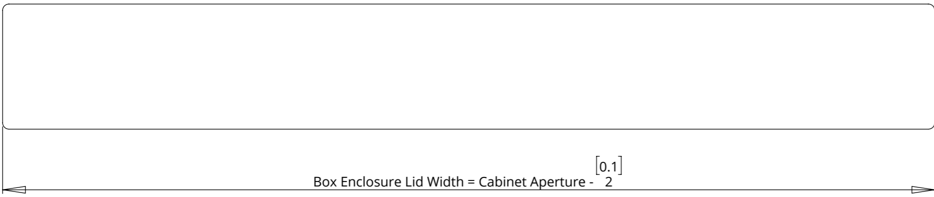
BOX ENCLOSURE LID (TAPERED) - TOP VIEW
